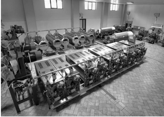
Figure 7.5 Virgin olive oil extraction plant equipped with plural malaxing machines in parallel. Photography courtesy of Alfa Laval Olive Oil S.p.A.
